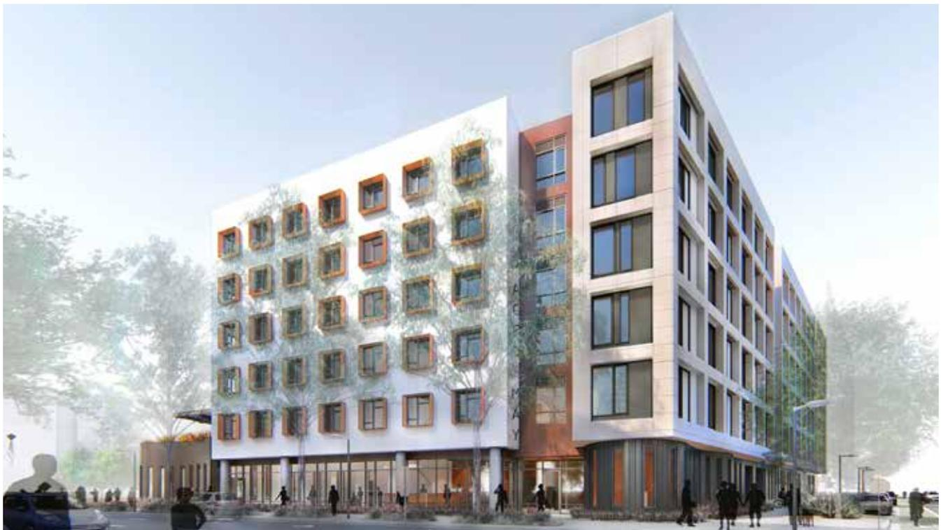
Maceo May, a 105-unit, all-electric residential development in San Francisco, is designed with an energy recovery ventilator with a MERV 13 filter, operable windows, and ceiling fans for every residential unit as well as a community space powered by on-site solar to maintain indoor air quality and continue operations during wildfires, heat waves, and power outages. Read more at [developingresilience.uli.org/](https://developingresilience.uli.org/).
